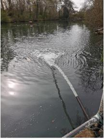
As can be seen from the photos on the left the pump, in conjunction with a special venturi on the outlet hose, quickly reoxygenates large volumes of water. Typically, we run the pump for around 4 hours at a time with around 144,000 litres of water being oxygenated. The pump is used in different locations around the Loch each time it is used.
